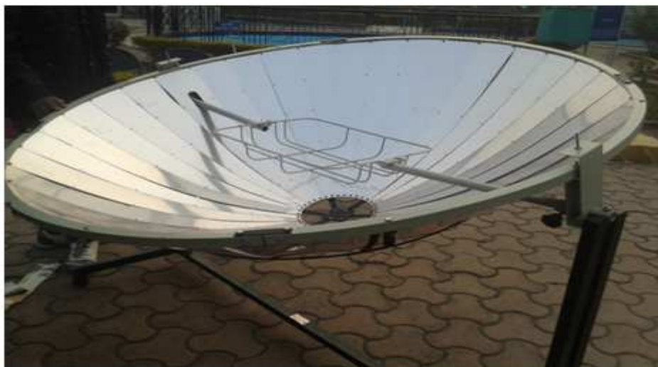
Figure 1a: Solar Dish Arrangement
